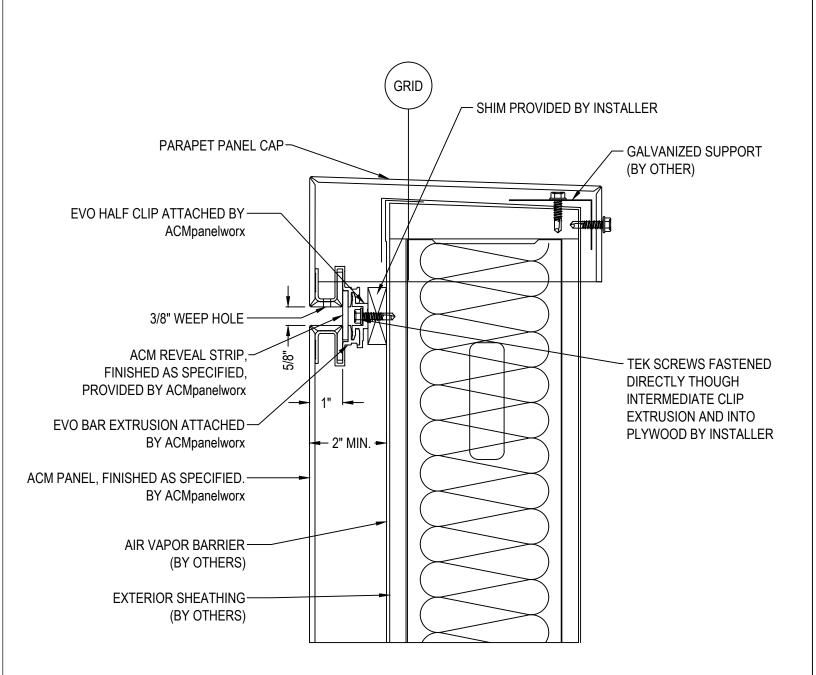
**O2 PARAPET CAP ALTERNATE DETAIL**
