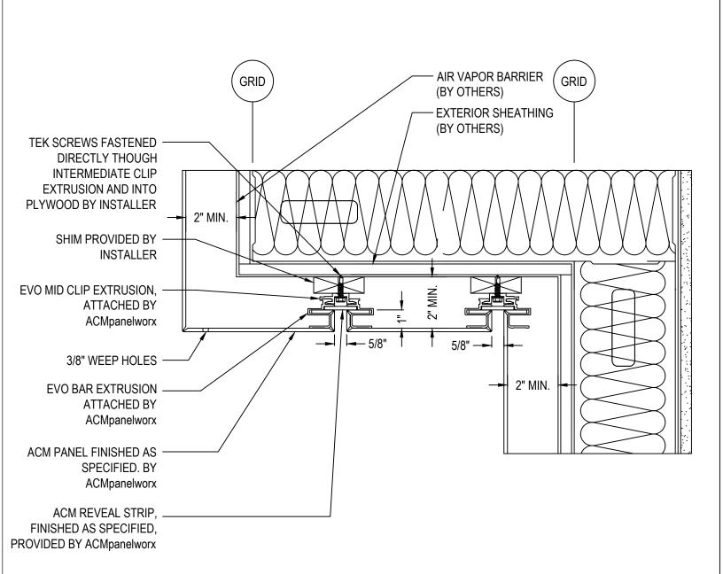
I O SOFFIT DETAIL
