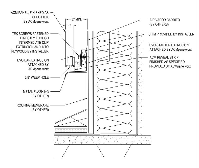
03 BASE TRANSITION AT ROOF TO WALL DETAIL
